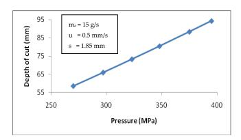
Fig.2 Water pressure versus depth of cut
