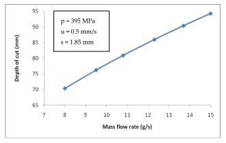
Fig.3 Abrasive mass flow rate versus depth of cut
