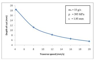
Fig.4 Nozzle traverse speed versus depth of cut
