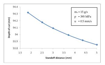
Fig.5 Standoff distance versus depth of cut
