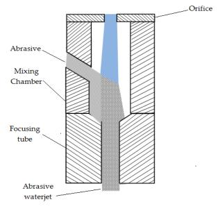
Fig.1 Abrasive injection nozzle
